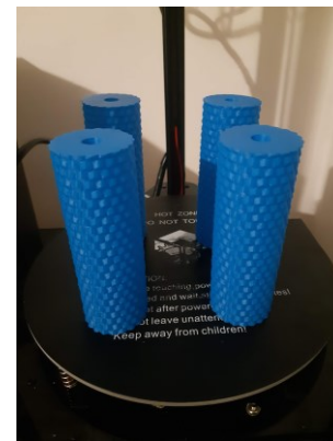
Image 2. Printed rollers on FDM 3D printer
