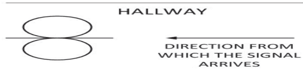
Fig. 9. Impact of the antenna radiation pattern is pronounced under waveguiding effect of hallway
