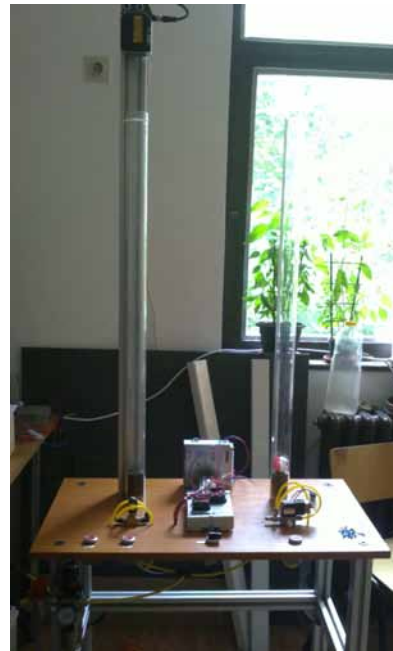
Fig. 1. Didactic model of servo pneumatic system.
