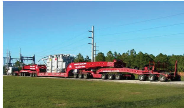
Sl.1. Transport transformatora
