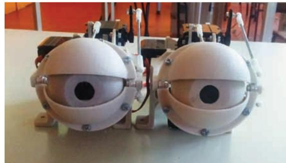
Figure 8. Assembled robotic eyes – frontal view
