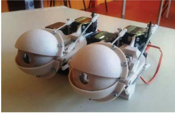
Figure 9. Assembled robotic eyes – isometric view
