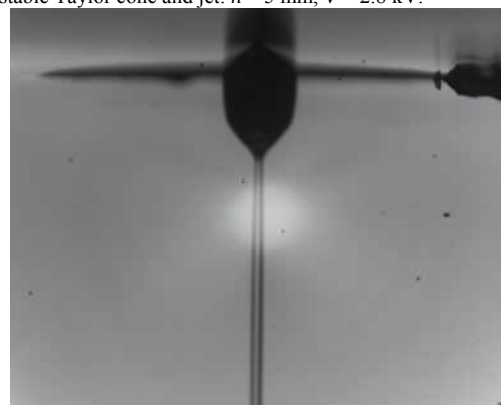
Fig. 5. Stable Taylor cone and jet obtained with setup no. 2: h = 7 mm, V = 5.5 kV
