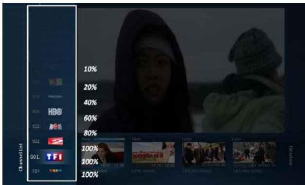
Fig. 2. Channel list – channels are represented by number and channel icon. Screenshot captured in moment of gradually appearing channel numbers and icons, from bottom to the top with a slight delay in between.
